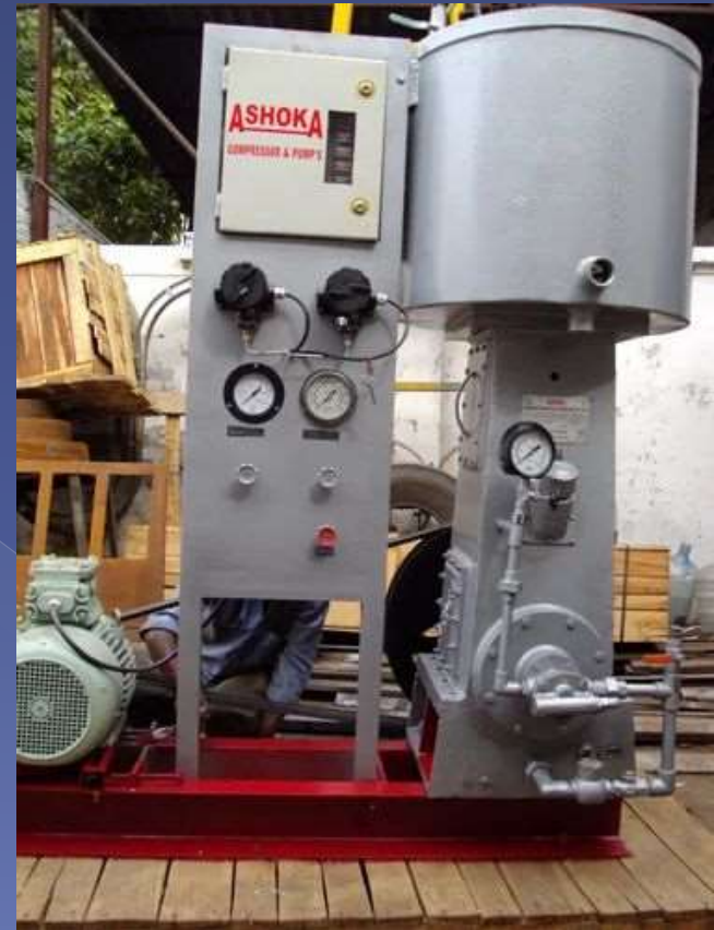
Oxygen Gas Compressors
