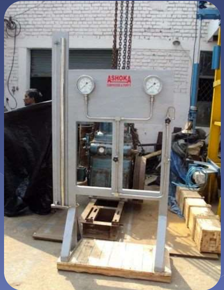
Cylinder Testing Station
