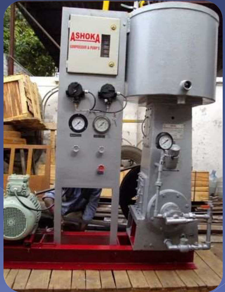
Nitrogen Gas Compressor
